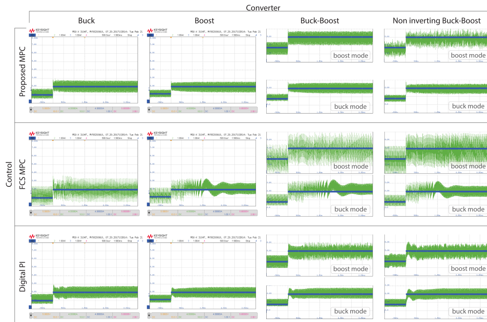
Fig. 8. Experimental dynamic responses using the proposed CCS-MPC, an FCS-MPC, and a digital PI as control.
